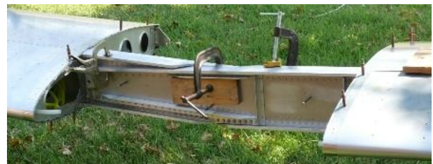
Lined up, Clamped, Ready to Drill
